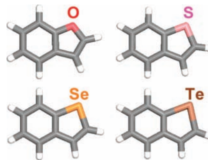
Figure 8. Optimized structures of the group 16 heterocycles (B3LYP/6–31+G* (3–21G** for the heteroatom)).
